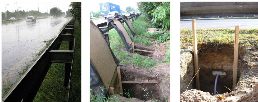
Fig. 1.9: Pictures of a rainfall event, sampling chamber and installed wick (from left to right).
