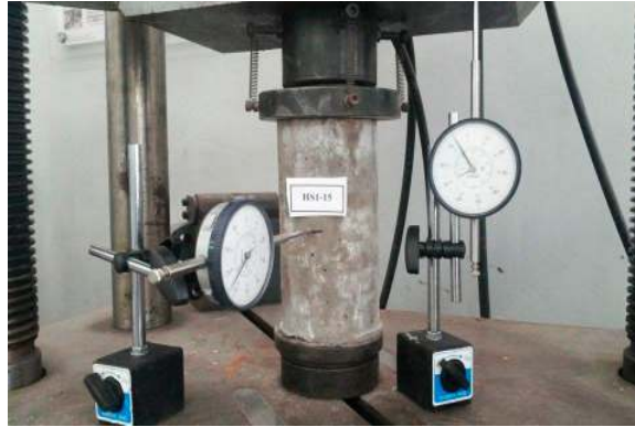
Figure 7. Experiment of Poisson's ratio and elastic modulus.
