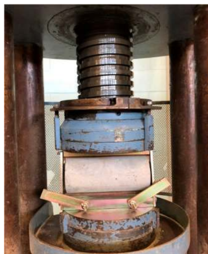
Figure 6. Splitting tensile test.
