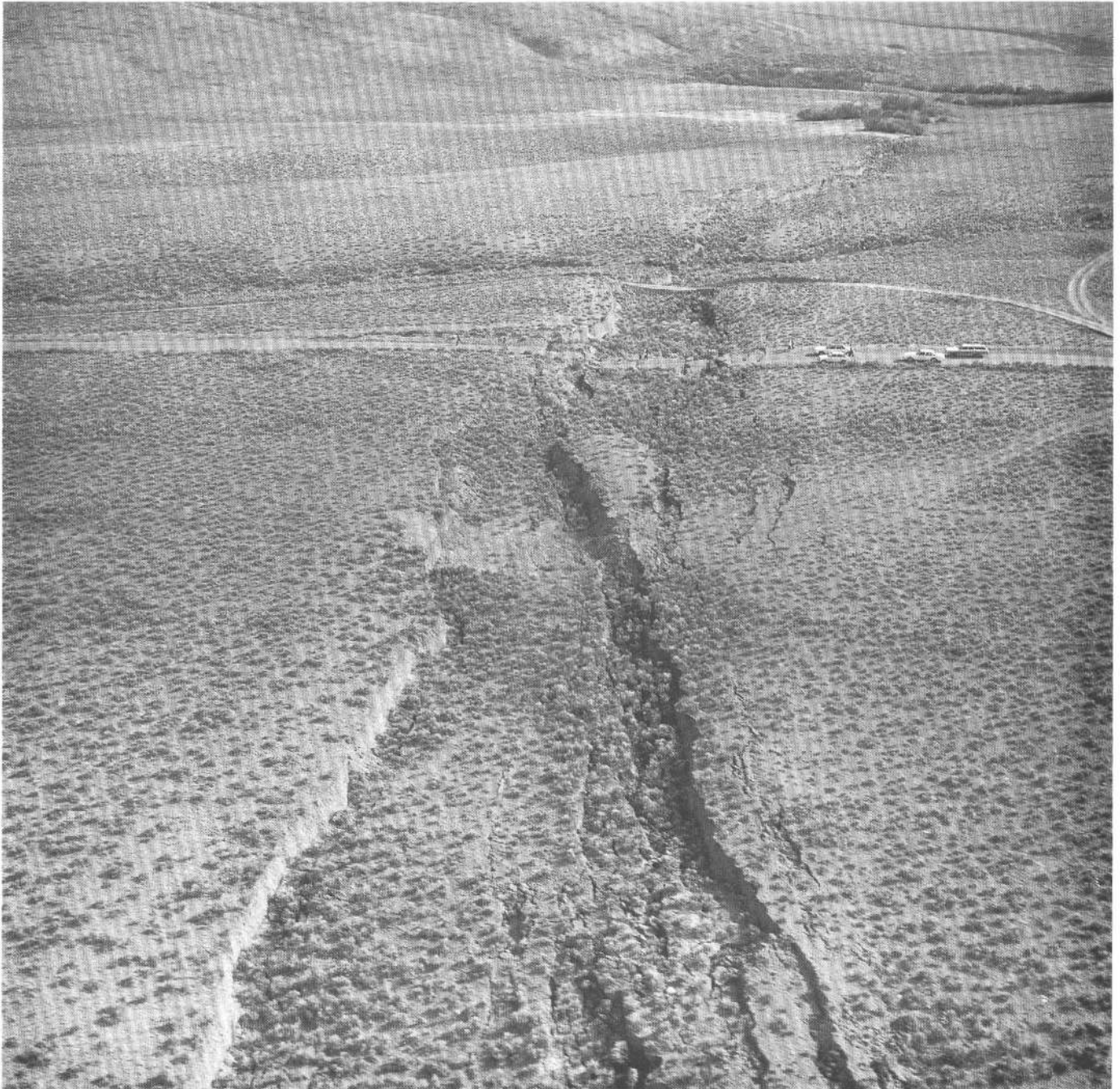
FIGURE 5.—Graben formed in the fault rupture of the 1983 Borah Peak, Idaho, earthquake.
