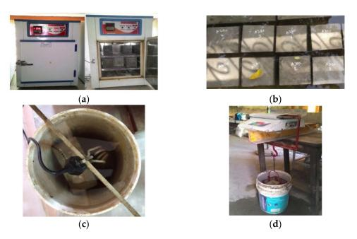
**Figure 4.** (a) Samples in oven drying; (b) samples immersed in water; (c) samples in boiling water; (d) Sample in apparent basket.
