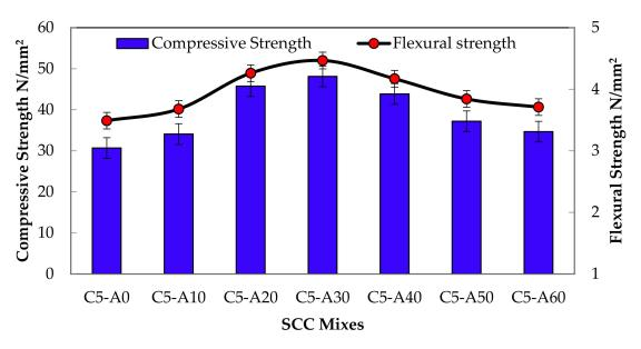
Figure 10. Compressive and flexural strength of SCC mixtures.
