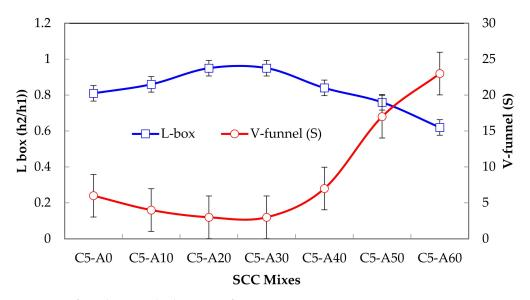
Figure 9. V-funnel time and L-box ratio of SCC mixtures.
