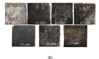
Figure 6. (a) Specimens immersed in  $MgSO_4$  solution and (b) specimens after immersion in  $MgSO_4$  solution.
