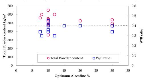
**Figure 14.** Interpretation between the optimum percentage of alcoofine with total powder content and the W/B ratio.
