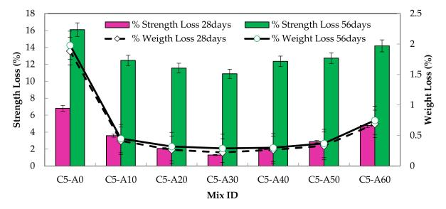
Figure 18. Percentage of strength and weight loss due to sulphate attack.
