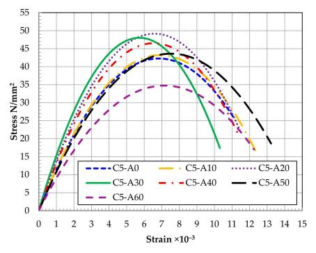
Figure 11. Stress-strain curves of SCC mixes with varying % of alccofine.
