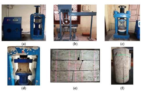
**Figure 3.** Testing of specimens in laboratory (**a**–**c**). Test setup of compression, flexure, and E-for concrete and (**d**–**f**) failure pattern of cube, prism, and cylinder.
