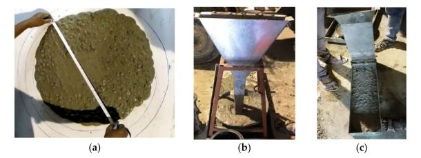
Figure 2. Testing fresh state of SCC in laboratory (a) slump flow, (b) V-funnel, and (c) L-box.
