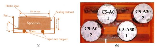
Figure 5. (a) Schematic procedure of sorptivity and (b) samples placed in the sorptivity pan.
