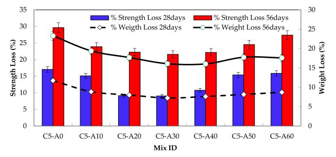
Figure 19. Percentage of strength and weight loss due to acid attack.
