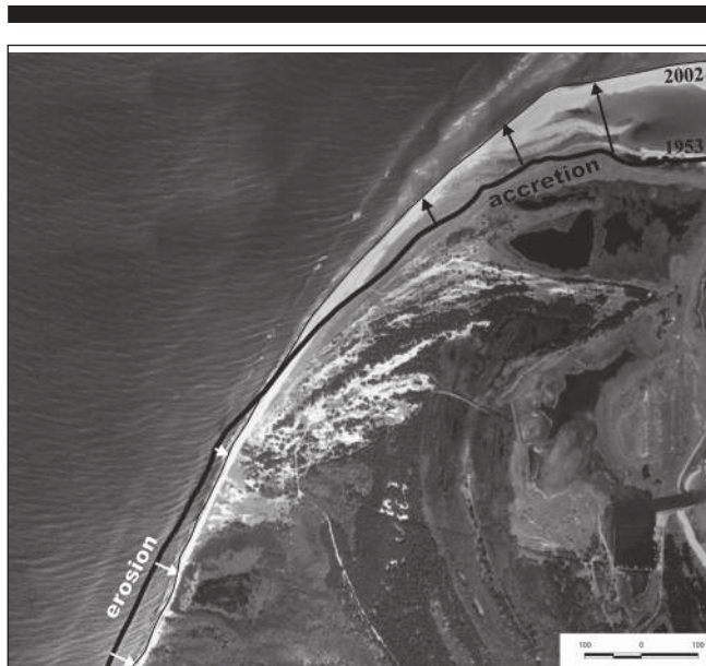
Figure 6. Aerial photograph of 2002, focusing in upon the northern part of the Darss Peninsula. The coastlines from 2002 and 1953 are shown, indicating clearly a change from erosion in the south to accretion in the north.
