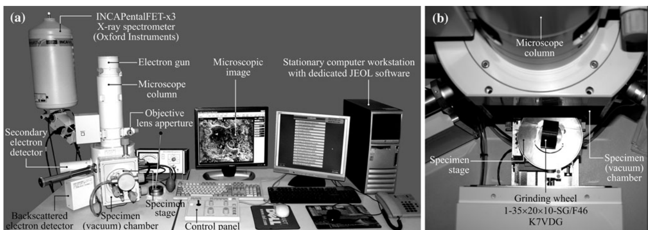
Fig. 1 The JEOL JSM 5500LV scanning electron microscope produced by JEOL Ltd.: a general view of microscope, b view of the grinding wheel prepared for assessment placed on the specimen stage
