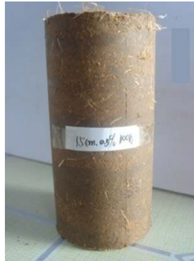
FIGURE 3: Sisal fiber-reinforced soil sample (fiber length of 15 mm and content of 0.5%).
