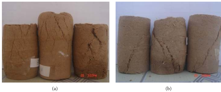
FIGURE 9: Fracture modes of the fiber-reinforced soil: (a) crack failure mode for soil reinforced with 15 mm long sisal fibers and (b) shear surface failure mode for soil reinforced with 5 and 10 mm long sisal fibers.
