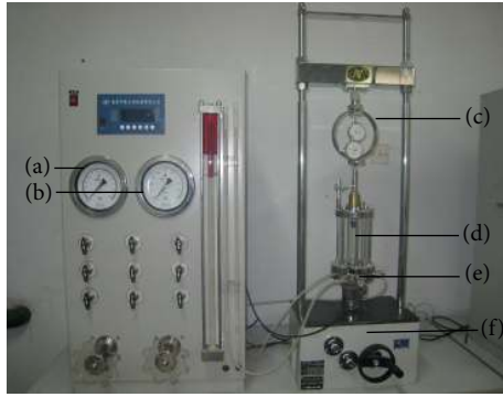
FIGURE 1: Triaxial shear test apparatus: (a) confining pressure gauge, (b) back-pressure table gauge, (c) proving ring, (d) pressure chamber, (e) pore water pressure sensor, and (f) testing machine.
