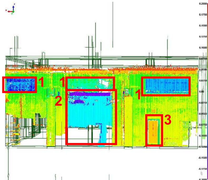
Figure 1. Deviation analysis compares points to the BIM or points to points. The figure illustrates a deviation analysis performed by comparing the points to a BIM. Problem regions found in the deviation map are highlighted by red rectangles. Regions 1 are unmodeled windows, region 2 is an indentation that was not modeled at the correct setback, and region 3 is a door that was modeled at the wrong location.
