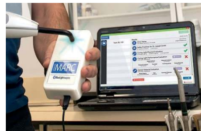
Figure 2. The radiant emittance values were recorded via spectrophotometric methods. (A) A laboratory-grade thermopile system. (B) A laboratory-grade integrating sphere spectrophotometer. (C) An in-office checkMARC portable spectrophotometer.
