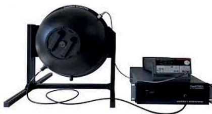
Figure 2. The radiant emittance values were recorded via spectrophotometric methods. (A) A laboratory-grade thermopile system. (B) A laboratory-grade integrating sphere spectrophotometer. (C) An in-office checkMARC portable spectrophotometer.
