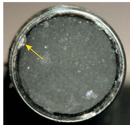
Figure 1. Contaminated and damaged light tips. (A) Light tip contaminated with resin composite and debris. (B) Damaged light tip by scratches, dents, and chipping.
