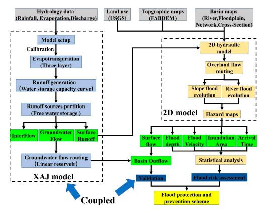
Figure 3. Flowchart of the coupled model.
