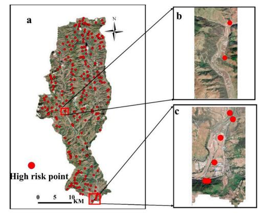
**Figure 12.** Maps of flood risk loci based on maximum water depth: (**a**) all high risk points in the basin; (**b**) the zoomed-in views of the high risk points in the mid reach of the basin; (**c**) the zoomed-in views of the high risk points in the downstream of the basin.
