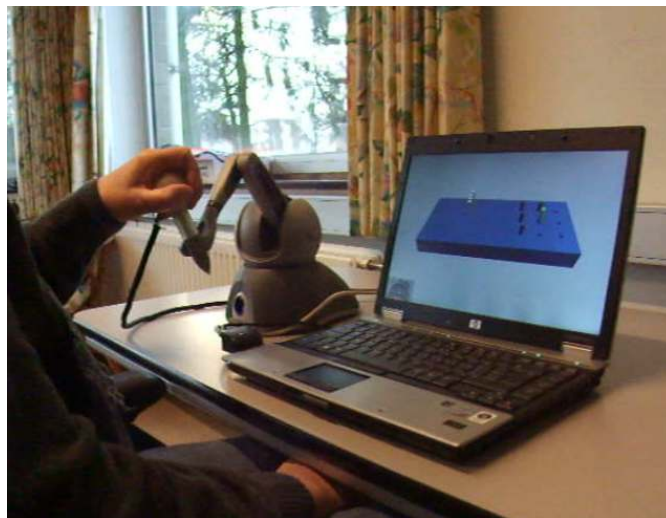
Fig. 1. MS patient performing the Virtual Peg Insertion Test. The setup is composed of a haptic device, an instrumented handle and a virtual reality environment. A computer placed in front of the user displays a virtual pegboard, a cursor representing the instrumented handle, and 9 virtual pegs.
