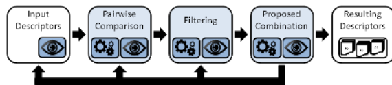
Figure 2: Schema of the descriptor selection process. Every step (blue) encompasses automatic data processing and visualization part. The input consists of many descriptors for one data set. These are compared and filtered resulting in a proposed set of independent descriptors. This is an interactive, guided analysis process. Feedback loops allow the user to refine results on demand.
