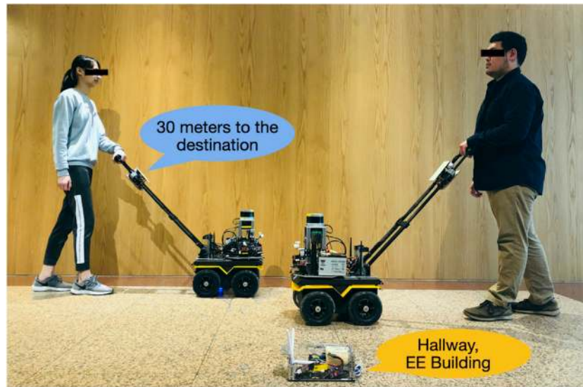
FIGURE 1 | Proposed navigation solution for BVI people. The designed system includes a guiding robot, an interactive harness, and UWB beacons. The system provides on-harness or on-beacon verbal semantic feedback. Usability studies were conducted to ensure that the designed guiding robot is easily accessible to BVI users.
