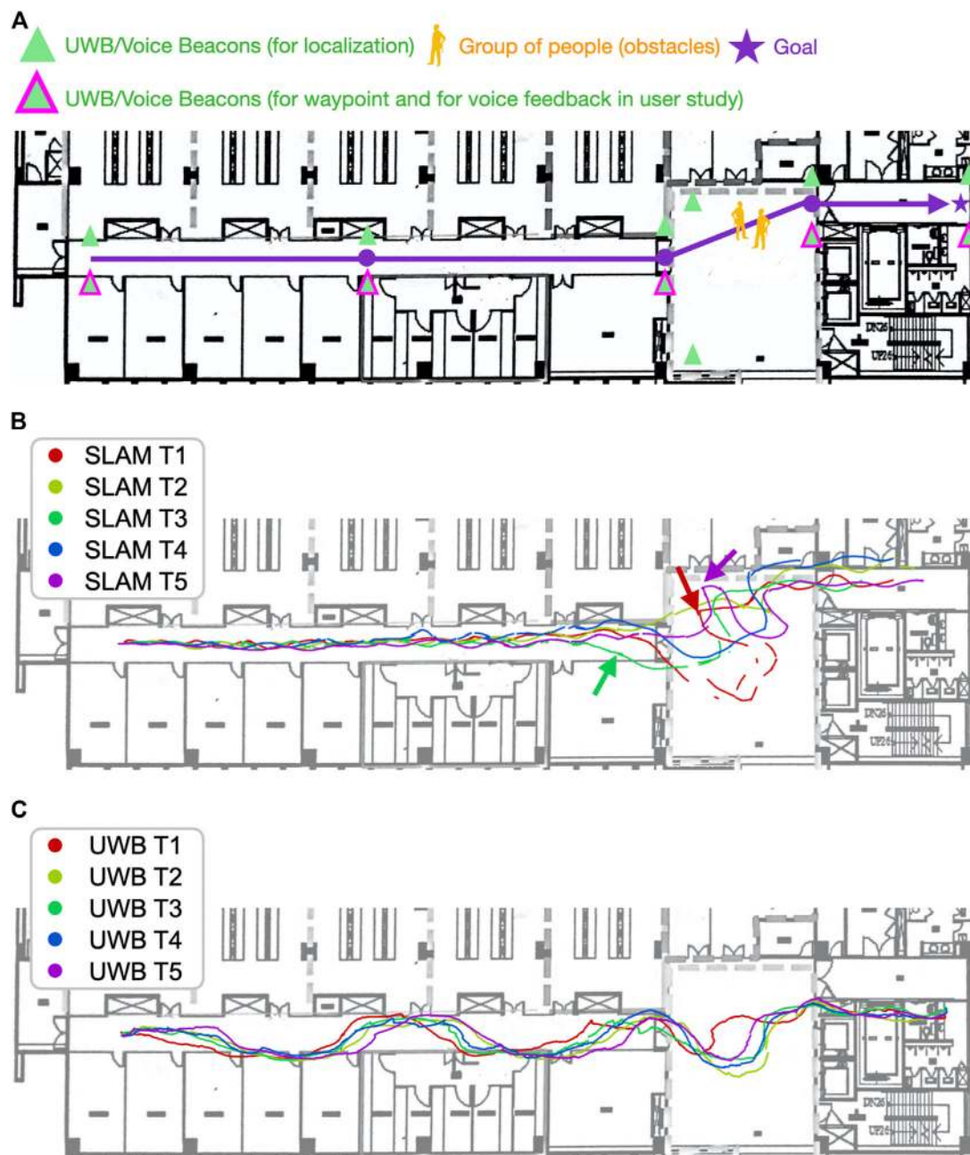
FIGURE 6 | Navigation with the SLAM algorithm in the dynamic environment was less stable and efficient than was navigation with the UWB beacons. (A) is the map with the UWB/Voice beacons and the designated route and waypoints. (B) visualizes the robot trajectories using proposed DRL with SLAM. (C) visualizes the robot trajectories using the proposed DRL with UWB localization. When using the SLAM algorithm, the robot tended to navigate to the right with an unnecessary loop and become trapped periodically (the red and purple arrows). The movement of pedestrians caused the SLAM algorithm to incorrectly estimate the distance traveled in a long corridor. The robot locations estimated by the algorithm (the green arrow) were different from the ground truth. Different results were obtained in the trials conducted with the SLAM algorithm, whereas consistent results were obtained in the trials conducted with the UWB beacons.
