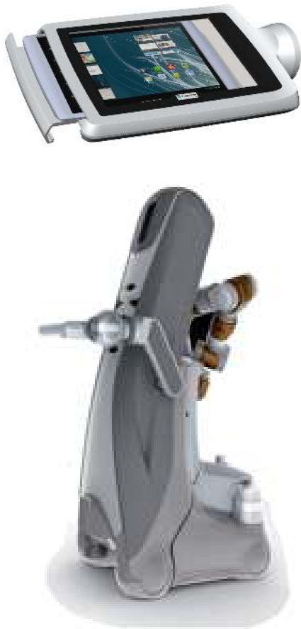
Figure 13. Design Drawings of the new tray kinematics with 3 degrees of freedom that allows height adjustment of the tray and switching between tablet pc and object placement
