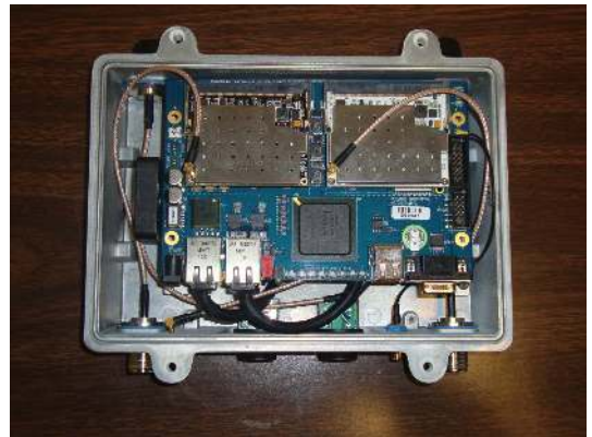
Fig. 4. Gateworks 2358 with Ubiquiti XR2 and XR5 Radios.
