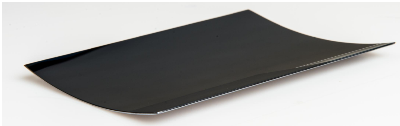
Figure 1. The basic element of our mirror technology: a mirror segment. Its typical dimensions are 100 mm by 100 mm by 0.5 mm, made of mono-crystalline silicon. A typical X-ray mirror assembly is composed of many thousands of mirror segments of many different mathematical prescriptions like this one, coated, aligned, and bonded together.
