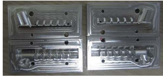
FIGURE 8: Fabricated convex and concave mold parts of AFPA.
