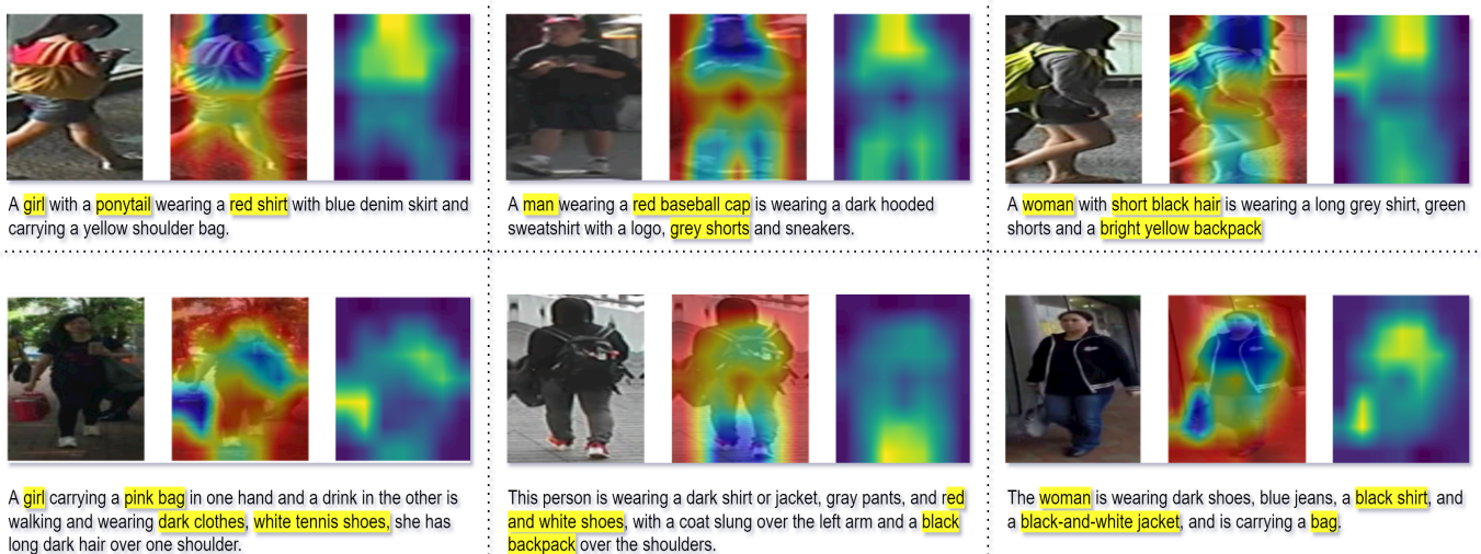
Fig. 5. Instance examples with saliency through the attention maps. For each group, the leftmost image is the raw pedestrian image, followed by the heat map of attention in the middle, and the highlighted areas in the right one represent the attentive saliency information.
