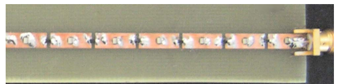
FIG. 1. (Color online) Photograph showing six periods of the nonlinear left-handed transmission line used in our experiments.
