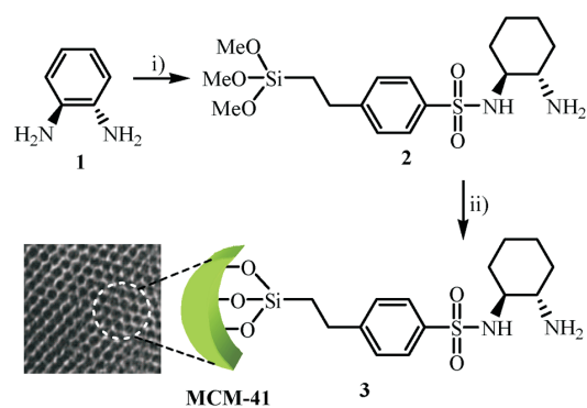
Scheme 1 Preparation of the MCM-41-supported chiral ligand 3
