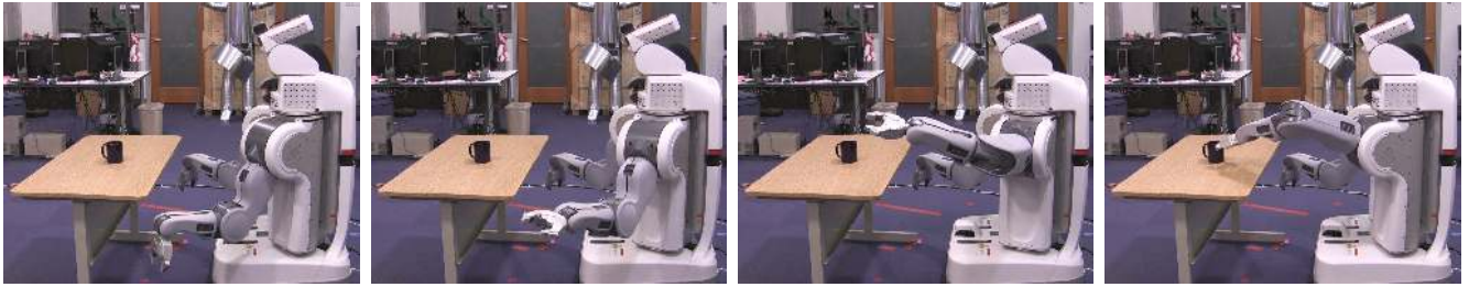
Fig. 2. The planner is tasked with finding a collision-free solution from (left) an initial pose in which the arm is under the table to (right) the goal pose.
