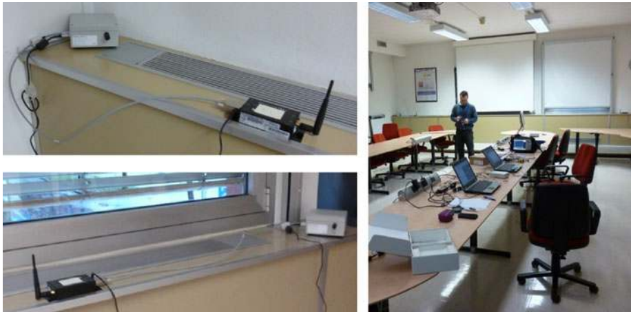
Figure 6. Different views of the large (5 m × 10 m) meeting room used for testing asynchronous pseudolite approaches. Four pseudolites were placed in the corners of the room.
