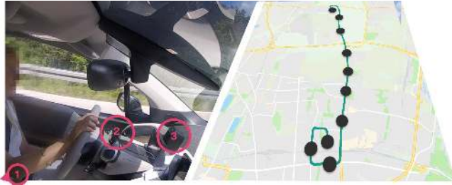
Figure 3: Left: the voice interface was controlled by a wizard on the backseat (1), two cameras streamed data to an emotion recognition software and provided the wizard with a view of the instrument cluster (2), the voice feedback was output through loudspeakers (3). Right: Experiment route. Map data ©2018 GeoBasis-DE/BKG, map view ©2009 Google
