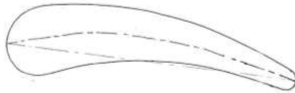
Figure 6. The Cambered – Cambered Aerofoil Drawn in Full – Size Dimensions
