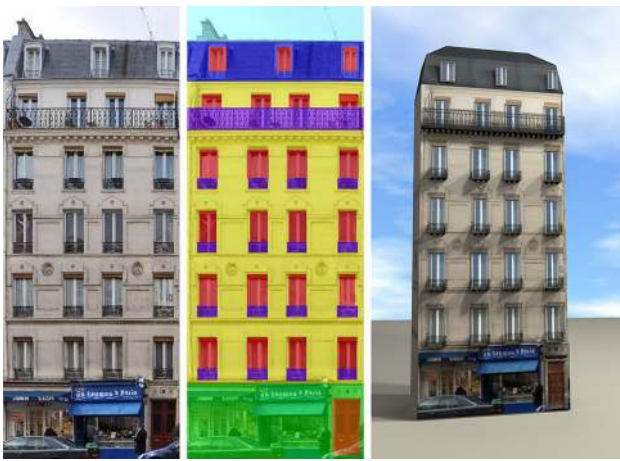
Fig. 1 The input to our system is cropped and rectified facade image ( left ). We process the image by our three layers to produced a labeled output image ( middle ). From this output we produce a textured procedural model ( right )
