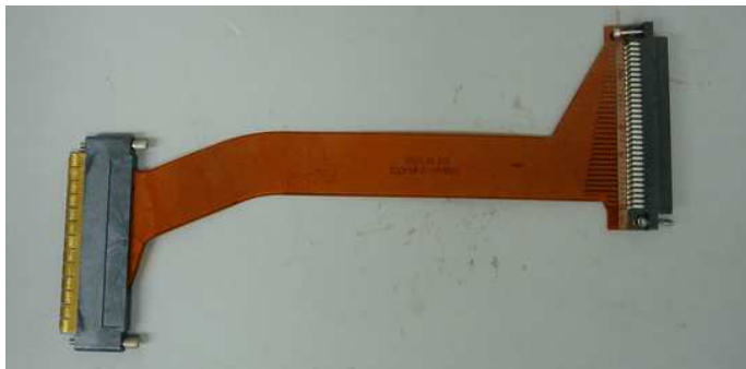
Figure 37. Photograph of a warm cable used to connect the calorimeter signals from the feedthrough pin carriers to the FEB inputs via the baseplane.
