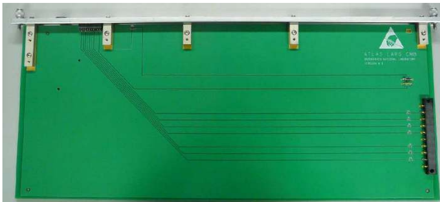
Figure 34. Photograph of a CMB. The output connector to the ELMB is visible in the upper left.
