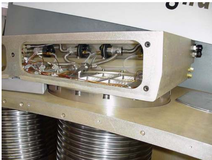
Figure 38. Photograph of a pedestal installed on a detector mockup, with no warm cables installed. The vacuum lines and pneumatic valves are visible inside the pedestal.
