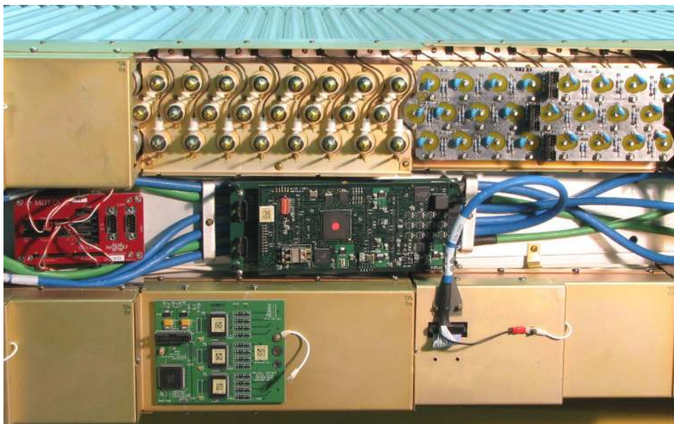
Figure 4. A photograph of the readout end of an end-cap MDT chamber where the assembly has been staged in sections to illustrate the tube ends with gas tubelets visible (upper center), one hedgehog board attached to the tube ends (upper right), one mezzanine board plugged through the inner Faraday cover (lower left), and a completely enclosed mezzanine board (lower right). In the center is the “chamber service module” (CSM) without its protective cover, and the red box to its left contains an “embedded local monitoring board” (ELMB).
