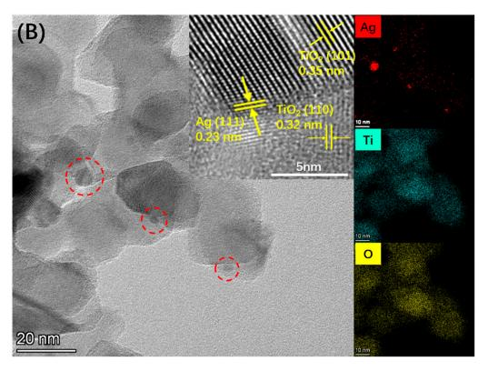
**Figure 1.** HR-TEM images and EDX mappings of (**A**) the L-Ag/TiO<sub>2</sub> and (**B**) the S-Ag/TiO<sub>2</sub> (red circles label the Ag nanoparticles).
