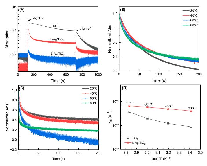
**Figure 5.** (**A**) Absorption changes of the three samples at 1550 nm before and after 375 nm laser irradiation in N<sub>2</sub> atmosphere at room temperature; normalized optical absorption relaxation of the undecorated TiO<sub>2</sub> (**B**) and L-Ag/TiO<sub>2</sub> (**C**) in N<sub>2</sub> atmosphere. (**D**) Temperature dependences of the optical absorption relaxation kinetic constant  $k_{et}$  in N<sub>2</sub> atmosphere for the undecorated TiO<sub>2</sub> and L-Ag/TiO<sub>2</sub>.
