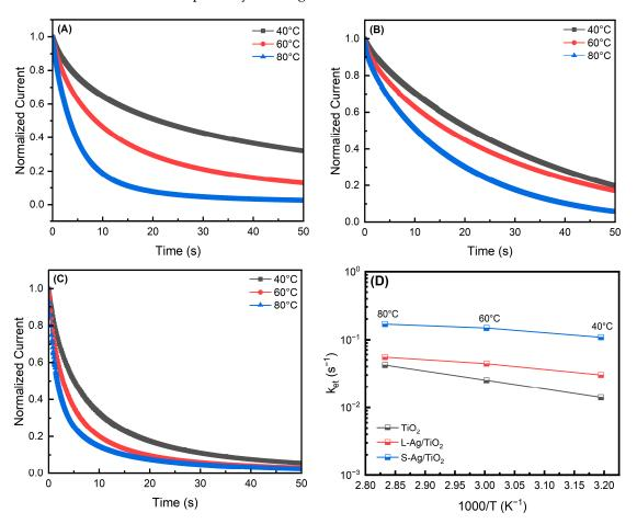
**Figure 3.** Normalized photocurrent relaxations of the undecorated TiO<sub>2</sub> (**A**), L-Ag/TiO<sub>2</sub> (**B**), and S-Ag/TiO<sub>2</sub> (**C**) in pure N<sub>2</sub> atmosphere. (**D**) Temperature dependences of the conductance relaxation kinetic constant  $k_{et}$  in N<sub>2</sub> atmosphere.
