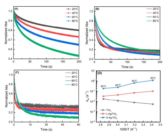
**Figure 6.** Normalized optical absorption relaxations of the undecorated TiO<sub>2</sub> (**A**), L-Ag/TiO<sub>2</sub> (**B**), and S-Ag/TiO<sub>2</sub> (**C**) in N<sub>2</sub> atmosphere containing methanol. (**D**) Temperature dependences of the optical absorption relaxation kinetic constant  $k_{et}$  in methanol atmosphere.
