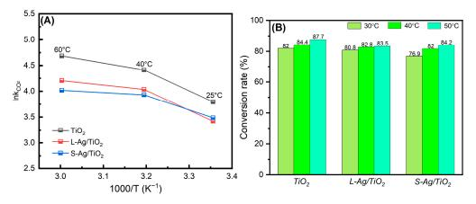
**Figure 8.** (**A**) Temperature dependences of the kinetic constants of the CO<sub>2</sub> generations for acetone oxidations. (**B**) Isopropanol conversions of the undecorated  $TiO_2$ , L-Ag/ $TiO_2$ , and S-Ag/ $TiO_2$  at different temperatures.
