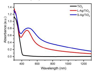
Figure 2. UV–Vis–NIR absorption spectra of the undecorated TiO<sub>2</sub>, L-Ag/TiO<sub>2</sub>, and S-Ag/TiO<sub>2</sub>.
