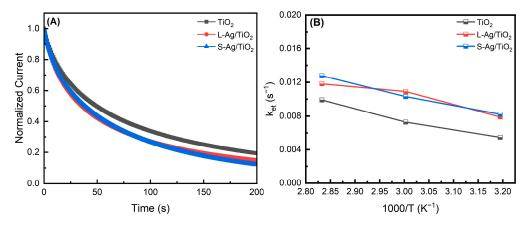
**Figure 7.** (A) Comparison of current relaxations of the undecorated TiO<sub>2</sub>, L-Ag/TiO<sub>2</sub> and S-Ag/TiO<sub>2</sub> under vacuum at 80 °C. (B) Temperature dependencies of the kinetic constant  $k_{et}$  of the current relaxations.
