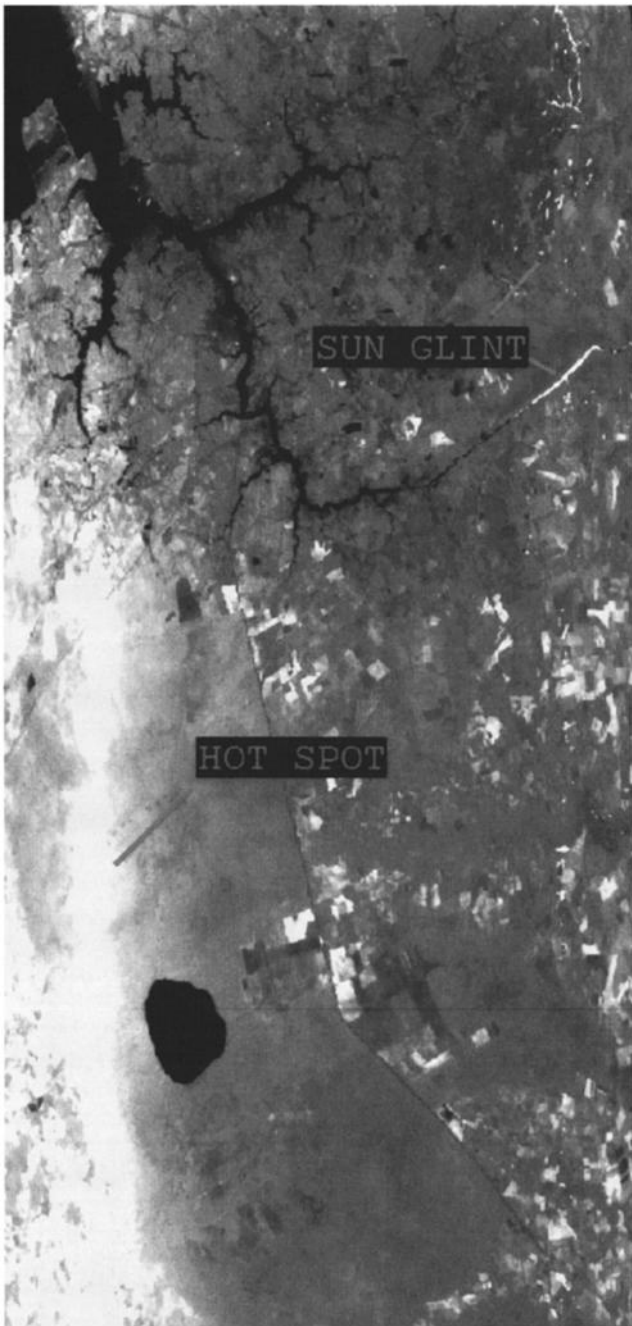
Figure 8b. Grey level image of the MAS scene ( 0.87 \mu\text{m} ) used in the BRDF inversion (Figure 8c and 8d). Annotations on the images point to the forest hot spot and water sun glint features.
