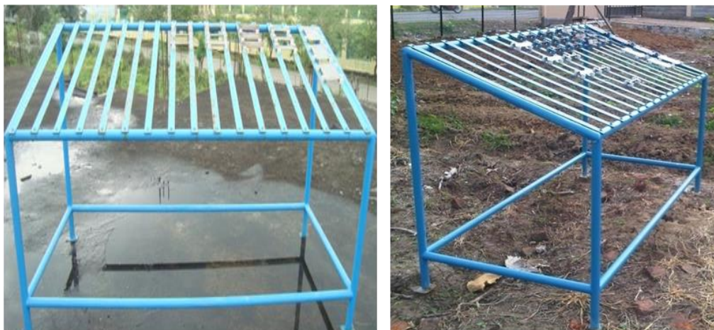
Figure 3. Specimens under exposure mounted on the rack.
