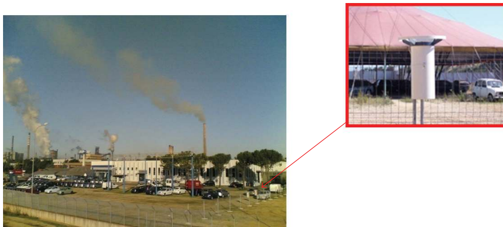
FIGURE 1: Bulk deposition sampler positioned round the borders of an industrial site in Taranto (Italy).
