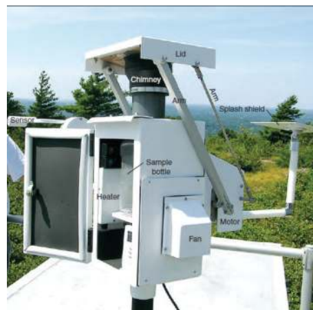
FIGURE 4: Newly designed wet-deposition sampler, Wet N-con System [195].
