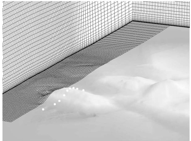
Figure 3: The Computational mesh. Only every second grid point is shown. The white dots denote the measuring stations located along line A.
