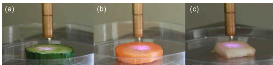
Fig. 1. (Color online) Plasma inactivation of (a) cucumber slice, (b) carrot slice, (c) pear slice.
