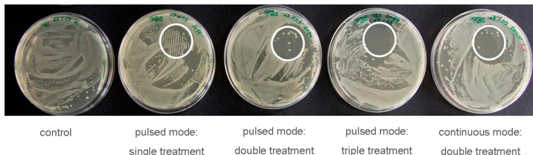
Fig. 4 Results of antibacterial treatment of E. coli on agar using different APPJ working modes as well as different treatment times [40].
