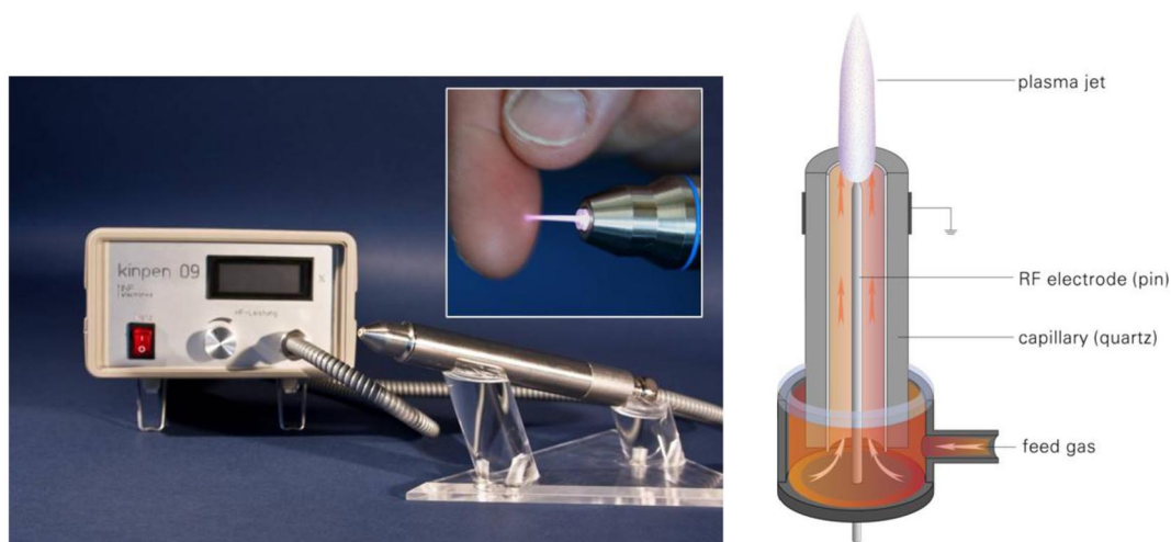
Fig. 2 Atmospheric-pressure plasma jet (APPJ; INP Greifswald, Germany) for experimental biomedical applications (left: CE approved device; right: schematic set-up) [40].
