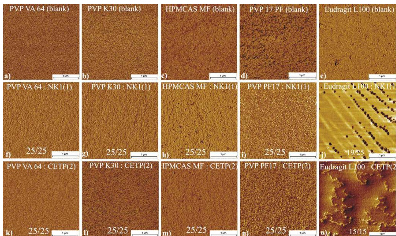
Fig. 4 Nanometer homogeneity is shown with phase maps recorded with tapping-mode AFM on fracture surfaces of the blank excipients ( a–e ), and corresponding combinations with NK1(1) ( f–j ), and with CETP(2) at the bottom ( k–o ). The numbers visible in the image rows ( f–j , and k–o ) relate the number of comparably structured places with the number of investigated places. The scale bars as shown throughout all images are the same and correspond to a length of 1 \mu\text{m} .
