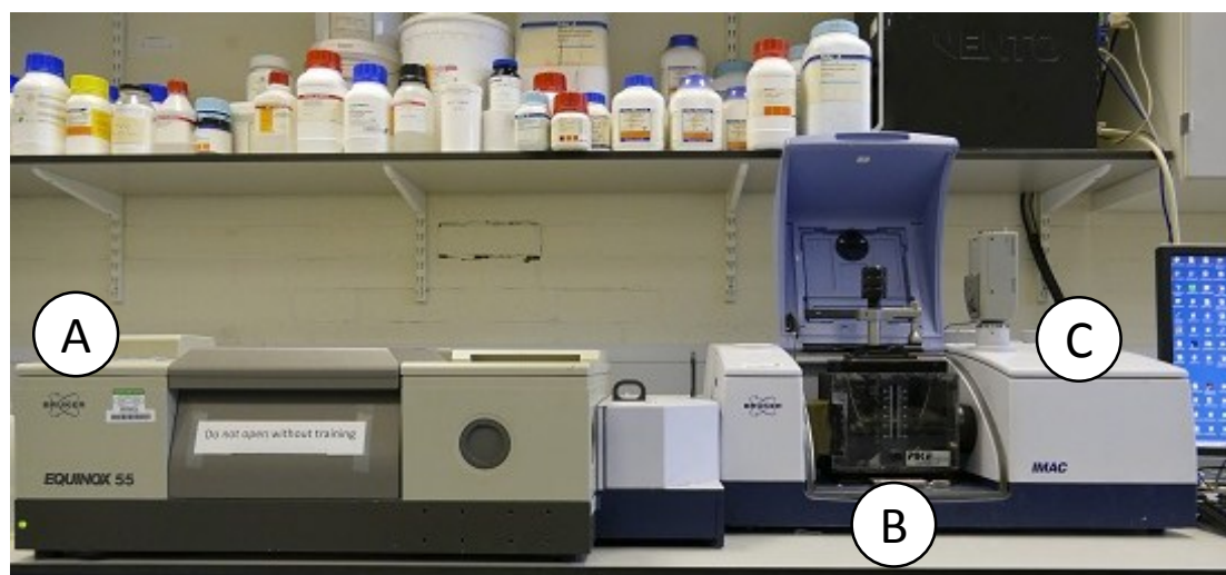
Figure 3.1 – Photograph of an FTIR spectroscopic imaging system that includes: (A) Bruker Equinox 55 FTIR spectrometer, (B) ATR accessory and (C) IMAC macrochamber.
