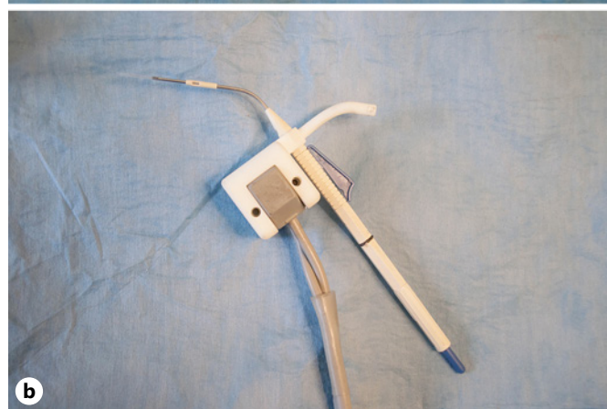
Fig. 1. Devices that allow coupling of the insertion tool to the robot. a Insertion tool mounted on the coupling device. b Coupling device attached to the FasTrak ® emitter and the insertion tool.
