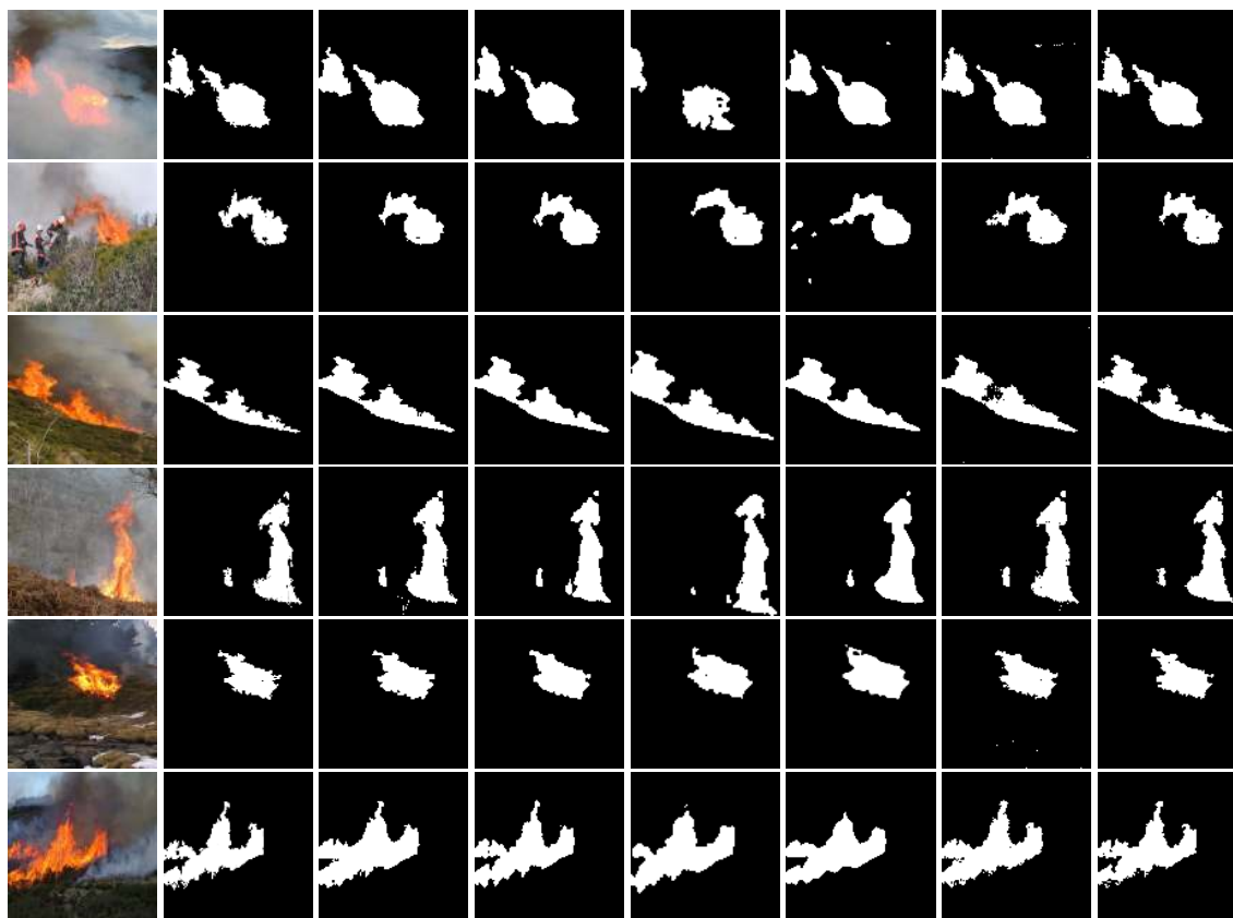
FIGURE 12. Visual comparison of various fire detection modules. From left to right: original fire images, ground truth, DenseNet, Attention U-Net, U-Net, SegNet, R2U-Net, and Ours, respectively.
