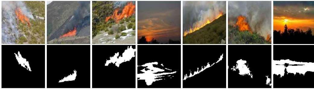
FIGURE 8. Results from trained segmentation module, up: original test images, down: segmentation results using the proposed segmentation framework.
