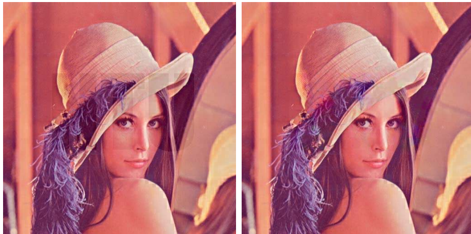
Figure 14. (a) The lena image (PSNR=31.37) embedded with the enhanced visible watermarking technique and (b) the recovered image (PSNR=35.80).
