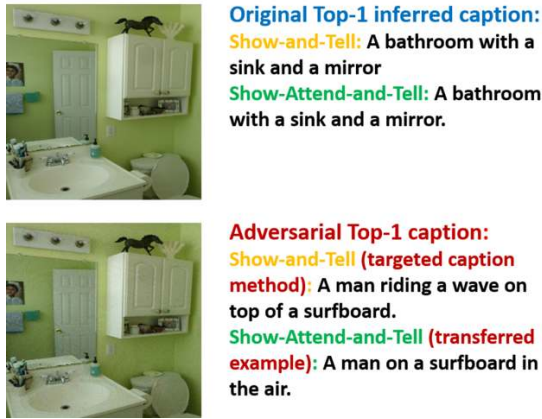
Figure 3: A highly transferable adversarial example ( \|\delta\|_2 = 15.226 ) crafted by Show-and-Tell targeted caption method, transfers to Show-Attend-and-Tell, yielding similar adversarial captions.
