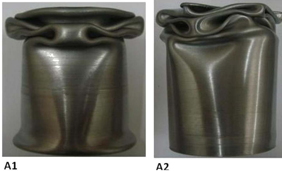
Fig. 8. Groove-less specimens after axial crushing.
