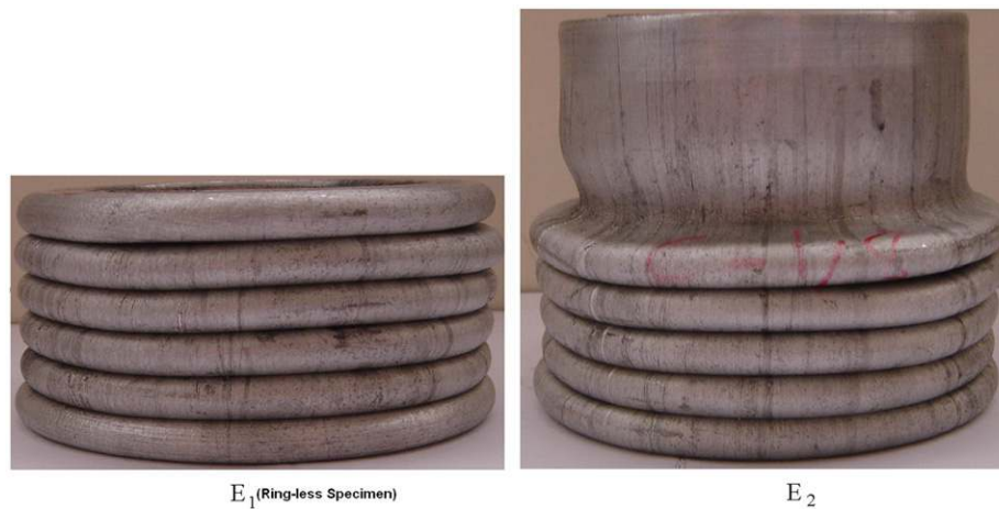
Fig. 3. Crushed shape of specimens of 200 mm length with expanding ring after quasi-static compression test.
