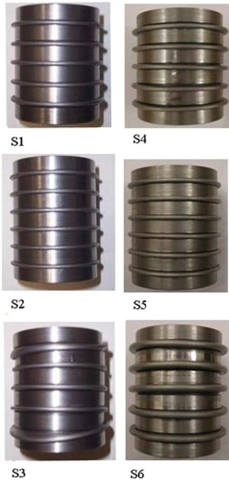
Fig. 9. Grooved specimens after axial crushing.
