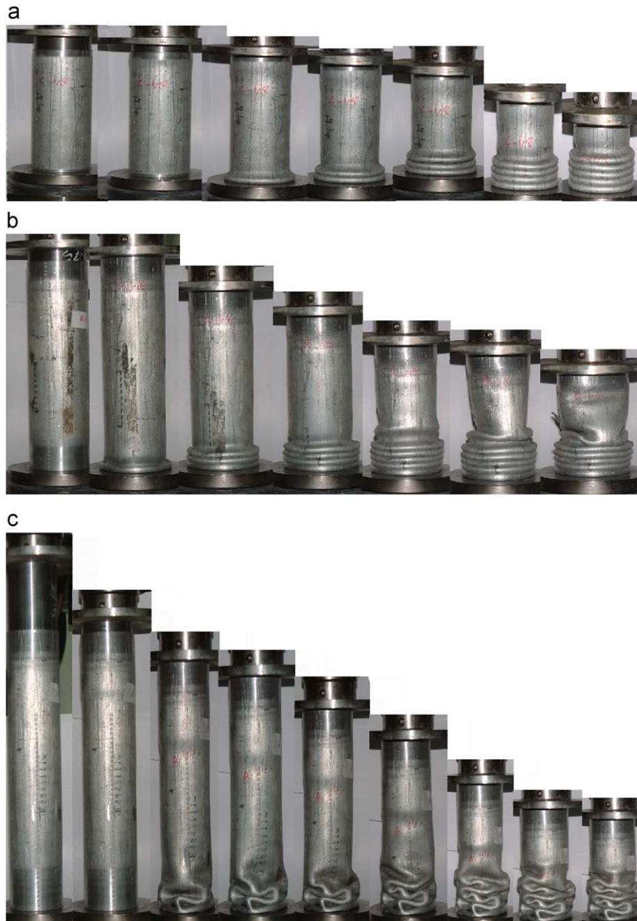
Fig. 11. Different stages of axial collapse of specimen (a) E2, (b) F2 and (c) G4.
