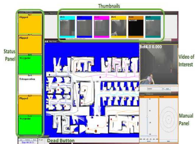
Figure 2. MrCS display in Open-queue: showing current conditions of all robots in the status panel (left-most window).
