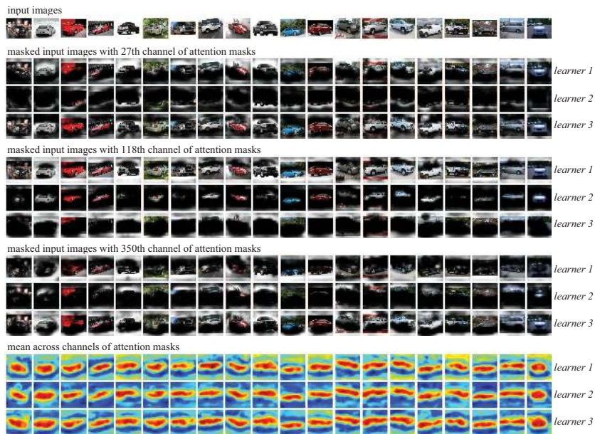
Fig. 6. The attention masks learned by each learner of ABE-8 on CARS-196. Due to the space limitation, results from only three learners out of eight and three channels out of 480 are illustrated. Each column shows the result of different input images. Different learners attend to different parts of the car such as upper part, bottom part, roof, tires, lights and so on
