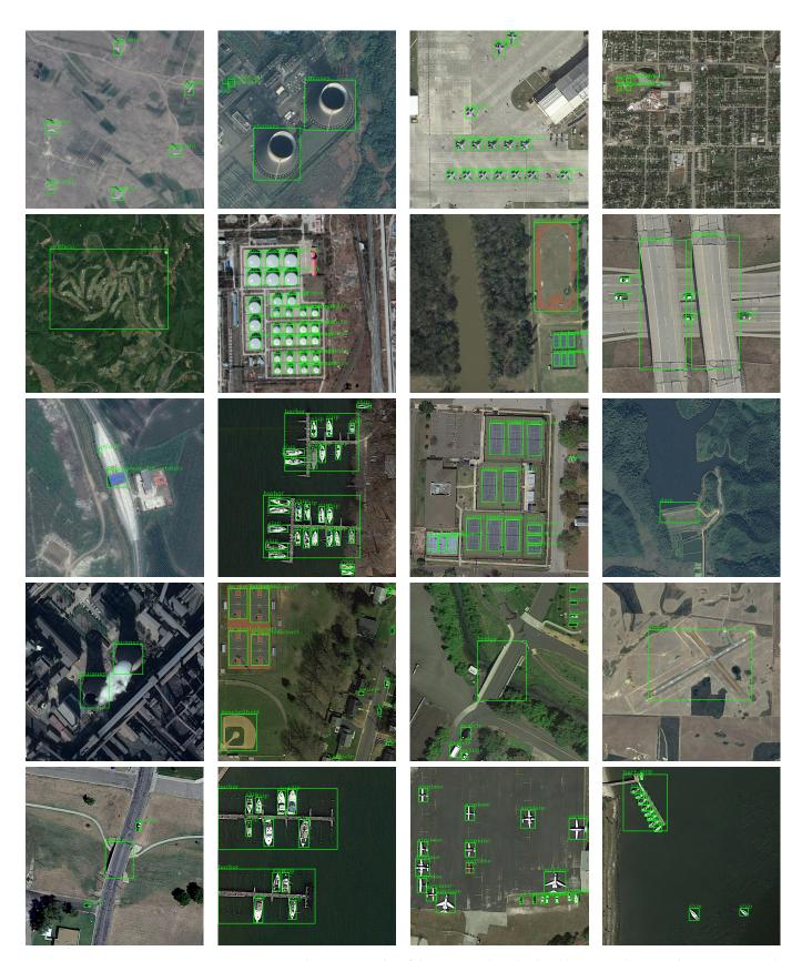
**Figure 8.** Some detection results of the proposed method on the DIOR dataset. The green rectangles represent TPs.
