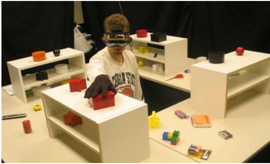
Figure 5. Test Environment: The user sat in the middle of test environment for the visual search task. It consisted of an omnidirectional workspace assembled from four tables each with 12 objects (6 primitive shapes and 6 general office objects) for a total of 48 target search objects.
