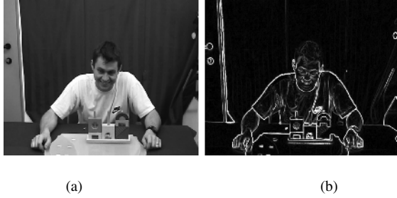
Fig. 5. (a) Grayscale image and (b) gradient strength image conducted from Sobel edge filters.
