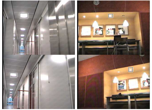
Fig. 6. Falsely matched ROIs (rectangles): in both cases, lamps are matched to a different lamp. Top: current frame. Bottom: frame from the database.
