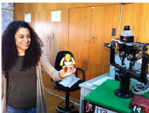
Figure 1. Joint attention in the context of social interaction with robots, using the Institute of Systems and Robotics' Integrated Multimodal Perception Experimental Platform (IMPEP). Hardware and motors for this platform were mounted within the scope of the Perception on Purpose (EC project number FP6-IST-2004-027268) project, and sensors were installed within the scope of the Bayesian Approach to Cognitive Systems project (EC project number FP6-IST-027140).
