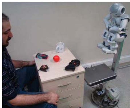
Figure 5. Experimental setting of the work by Yücel et al. [84] – reproduced by kind permission. To evaluate their method, several experiments were performed to model joint attention between a human experimenter (in the photo, on the left, co-author Cetin Meriçli is shown acting out the human experimenter's role) and an embodied agent. In this setting, the experimenter and the robot place themselves roughly 1.5 meters apart at opposite sides of a table, on which a number of objects are placed in a non-occluding fashion. A session of joint attention is initialised when the experimenter establishes eye-contact with the robot, which leads to a fully-frontal face image being acquired. The experimenter fixates his/her attention to one of the objects by looking at them in random order for a certain duration of time.
