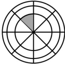
Figure 3. Example of a 2D shape context kernel with 24 bins ( n_r = 3 and n_\theta = 8 ).
