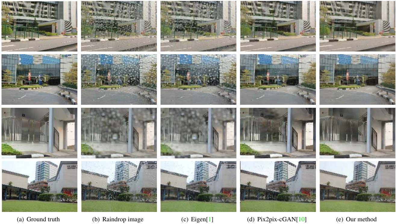
Figure 6. Results of comparing a few different methods. From left to right: ground truth, raindrop image (input), Eigen13 [1], Pix2Pix [10] and our method. Nearly all raindrops are removed by our method despite the diversity of their colors, shapes and transparency.
